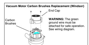
If armature commutator is grooved, extremely pitted or not concentric, the motor will need to be replaced or sent to a qualified service center.
